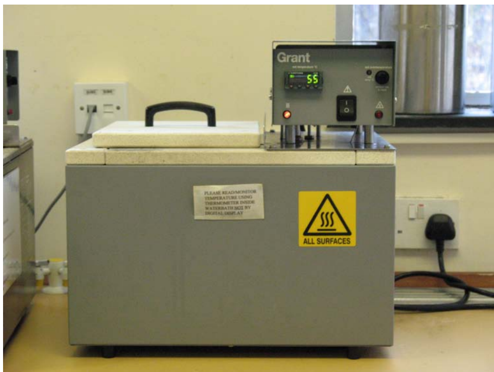
Figure 8: Oil bath in which the Olpidium brassicae resting spore filled capillaries were heat-treated
